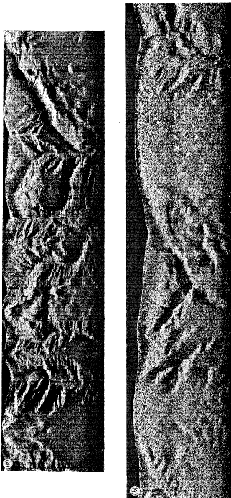
FIGURE 2. Sonograph views of canyons near the top of the continental slope on the Armorican margin (Belderson & Kenyon 1976). The 13 km (a) and 7 km (b) views are obtained by insonification downslope with a narrow beam sonar. Highlights indicate strong echoes. (a) Slope at 45\frac{1}{2}^{\circ} N, 4^{\circ} W intensely eroded by canyons. Length of trace, 54 km. (b) Slope at 48\frac{1}{2}^{\circ} N, 9\frac{1}{2}^{\circ} W with few canyons. Length of trace, 32 km.
